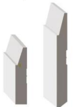
CHAMFERED CASING: 3 1/2" BASEBOARD: 5 1/4" (U)
